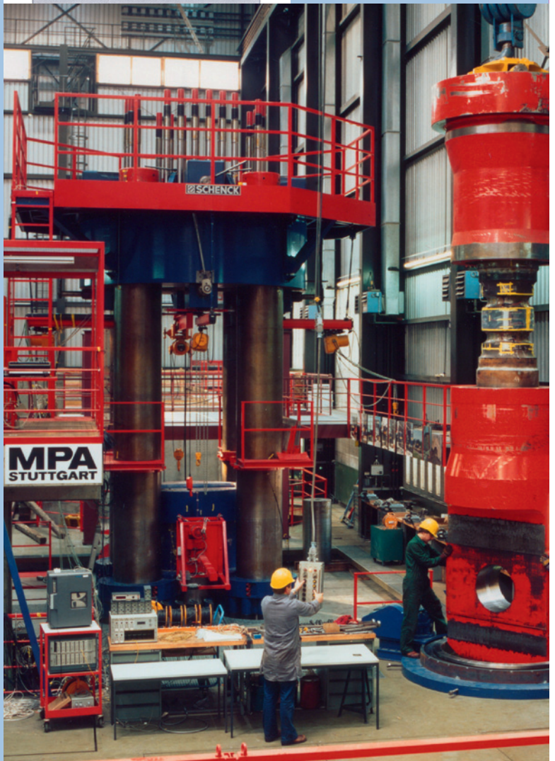
100 MN-Zugprüfmaschine: 100 MN Tensile Testing Machine MPA Stuttgart, Germany
